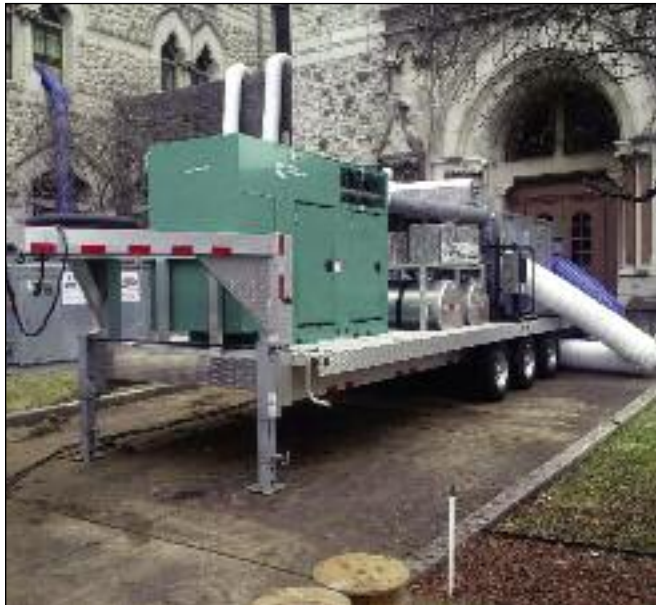
Trailer-mounted - MS-6000/5000 with heat recovery.
