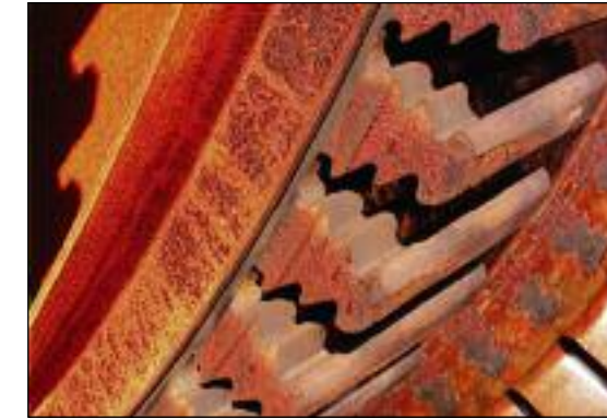
Deposits that contain chloride aggressively pit the turbine when it is allowed to sit in moist conditions. These pits become sites for corrosion fatigue. Courtesy: EPRI
